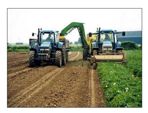
Here is the a harvesting machine. It lifts and separates the potatoes from the soil.
